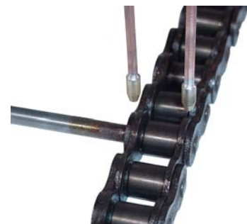
FORCING NOZZLES (after lubrication)
