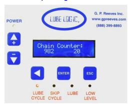
Shows POWER ON and unit in LUBE CYCLE with all but 20 segments of a 982 segment long chain already lubricated
